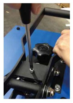
The screw maintain the arm to the elctromagnetic system for transport security reasons.
